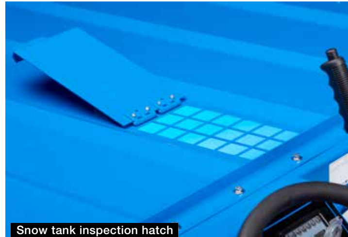
Snow tank inspection hatch
