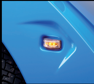
Turn signal front, rear and side
