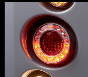
Tail lights Parking light & brake light
