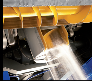
Screw conveyor wash system vertical
