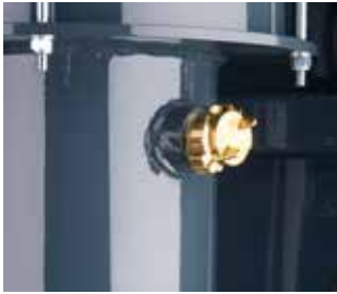
Screw conveyor wash system vertical
