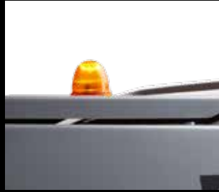
Flashing warning light
