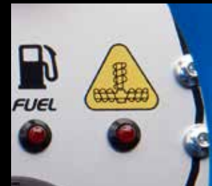
Conveyor screw overload warning system
